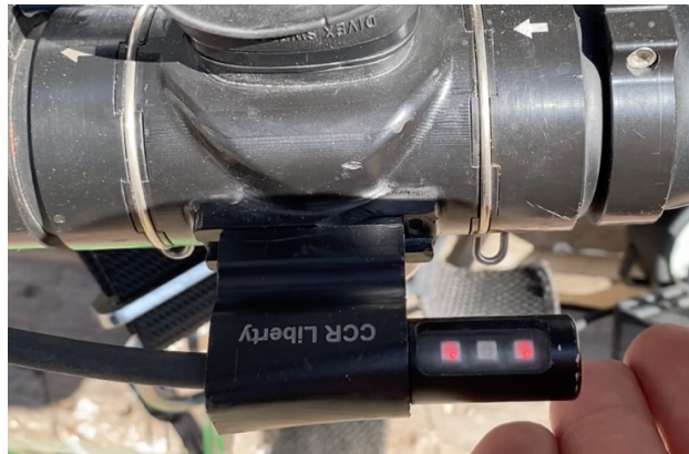
Both LEDs lit but in the shadow of the diver's hand
